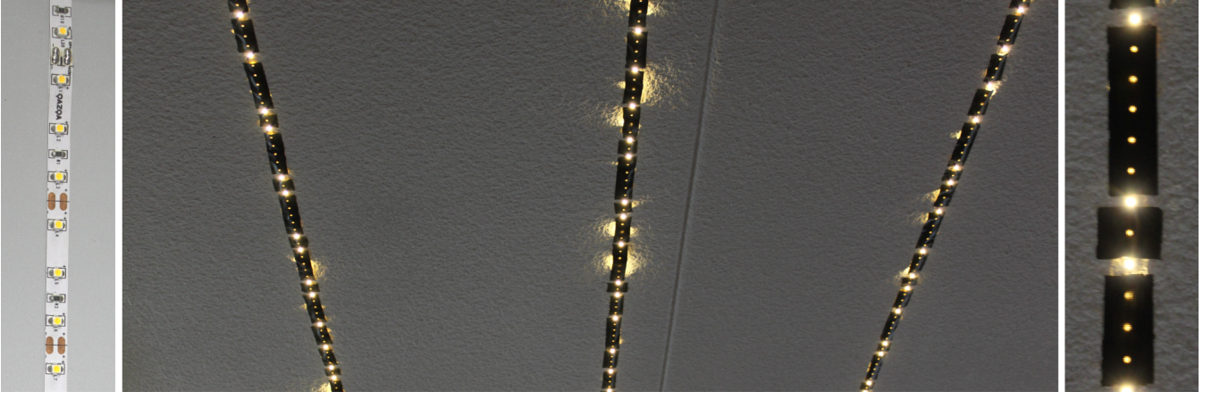
Figure 5: The LED setup. Left: The LED strips used in our setup. Middle: LED strips mounted to the ceiling, displaying the pattern used for decoding. Right: Detailed view of encoded LED strip.
