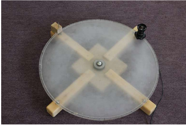
Figure 12: Setup for the rotating test. the camera movement is limited to one turning direction.
