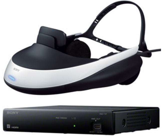
Figure 6: The Sony HMZ-T1 head mounted display, which was used in our prototype to allow the user to navigate a virtual world.
