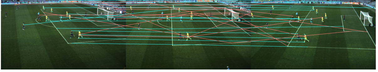
Figure 6: Example of multicamera feature matching using 3 cameras. All pairwise features are connected with each other using lines. Only a subset of the multicamera matches are shown, and the red mismatches will be removed later on in section 5.
