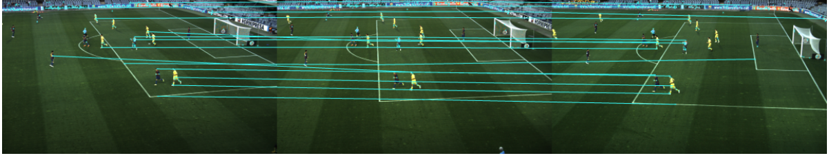
Figure 7: Multicamera feature matches, considered as inliers. Most outliers are removed using the angle-based filtering. Only a subset of the multicamera matches are shown.
