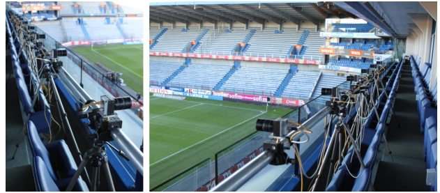
Fig. 2. Example of the camera line setup. Cameras are placed approximately one meter apart from each other. The distance to the field is about 20 meters.
