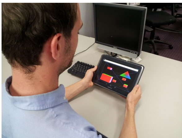
Fig. 9. Example of the mobile setup. Motion parallax is achieved on a tablet, using the front facing camera.
