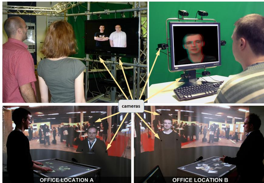
**Fig. 1** Restoring eye contact by synthesizing a virtual view in between the surrounding camera views.
