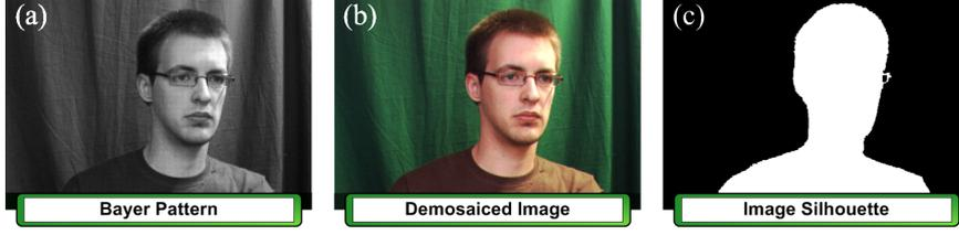
**Fig. 6** The preprocessing module performs demosaicing, undistortion and segmentation of the input images.
